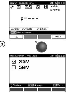
The meter is ready for measurement. The auxiliary display shows the value of the interference voltage and its frequency. The setting bar shows the measurement voltage, mains frequency set in the **MENU** and the distance between the electrodes.
