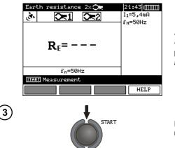
The meter is ready for measurement. The auxiliary display shows the value of the leakage current passing through the clamp and its frequency.
