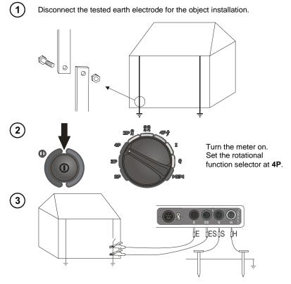
Connect the current electrode driver into ground to the **H** socket of the meter. Connect the voltage electrode driver into ground to the **S** socket of the meter. Connect the tested earth electrode to the **E** socket of the meter. Connect the **ES** socket to the earth electrode In question below the **E** cable. The tested earth electrode as well as the current electrode and voltage electrode should be aligned.
