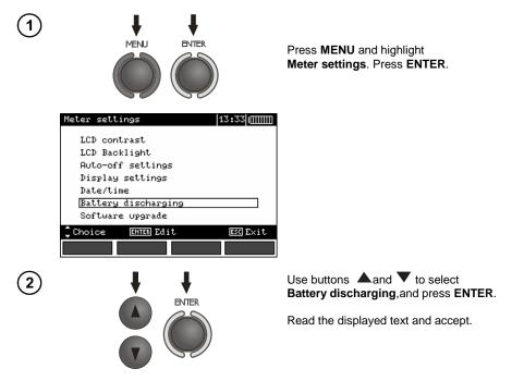
Discharging, which may last up to 10 hours depending on the level of the charge of the package, is signalled with the following message: **Discharging of accumulators in progress**.
