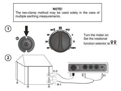
Connect the transmission clam to sockets H and E, while the measurements clamp should be connected to the clamp socket.
