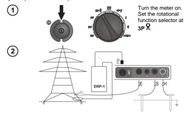
The current electrode (driven into earth) should be connected to **H** socket of the meter. The voltage electrode (driven into earth) should be connected to **S** socket of the meter. The tested leg of the pole should be connected to **E** socket of the meter with the lead. The tested leg of the pole, the current electrode and the voltage electrode should be arranged in one line.
