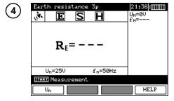
The meter is ready for measurement. The auxiliary display shows the value of the interference voltage and its frequency. The setting bar shows the mains frequency set in the MENU.
