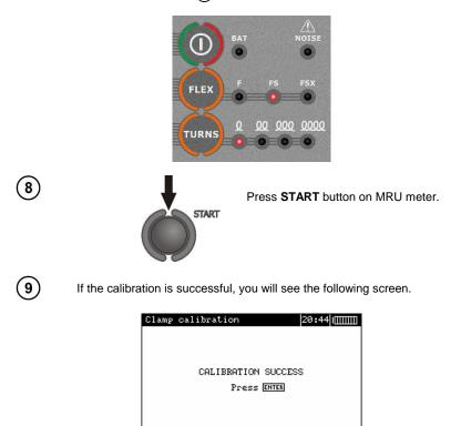
The meter has determined the correction factor for connected clamp. The factor is saved in the memory also when the power supply of the meter is off until the following successful calibration of the clamp has been performed.
