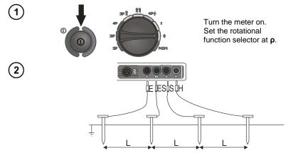
Connect the four aligned and equally spacer electrodes, which are driven into the ground, to the meter, and do so In accordance with the diagram above
