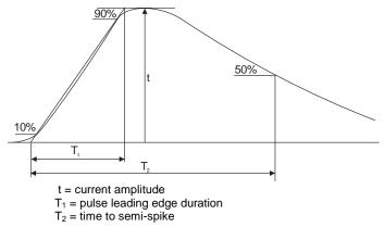
The pulse shape is determined by the relation  $T_1/T_2$  eg: 4/10 µs.
