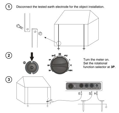
Connect the current electrode driver into ground to the **H** socket of the meter. Connect the voltage electrode driver into ground to the **S** socket of the meter. Connect the tested earth electrode to the **E** socket of the meter. The tested earth electrode as well as the current electrode and voltage electrode
