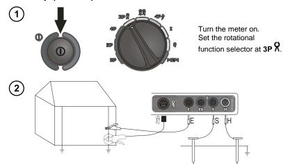
Connect the current electrode driver into ground to the **H** socket of the meter. Connect the voltage electrode driver into ground to the **S** socket of the meter. Connect the tested earth electrode to the **E** socket of the meter.
