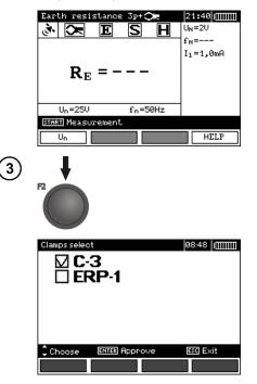
The meter is ready for measurement. The auxiliary display shows the value of the interference voltage and its frequency. The setting bar shows the mains frequency set in the MENU.
