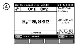
Read out the result. MRU-200-GPS The right side of the display shows the date, time and GPS coordinates.
