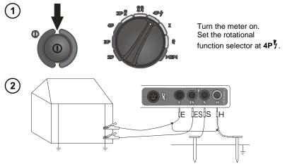
Connect the current electrode driver into ground to the **H** socket of the meter. Connect the voltage electrode driver into ground to the **S** socket of the meter. Connect the tested earth electrode to the **E** socket and the shield of the **H** cable.
