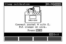
Connect ERP-1 adapter to the terminal of the clamps.
